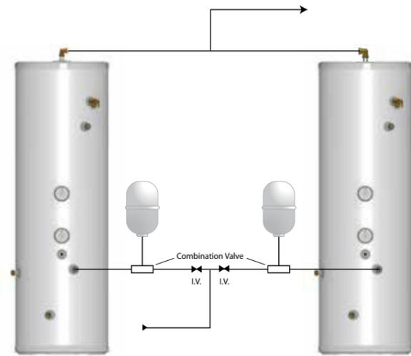
If two Thermstore cylinders are coupled together the secondary inlet and outlet pipes must be balanced. The units must be fitted on the same level.
