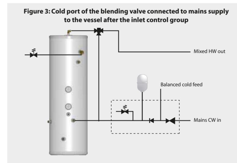
Figure 3 shows the cold port of the blending valve connected to the cold water supply to the vessel after the inlet control group. This should be the preferred method. It is recommended that the installer should ensure that there is no gravity circulation in the pipework connected to the cold port. If necessary, this can be achieved by fitting a non-return valve or using a thermal trap.
