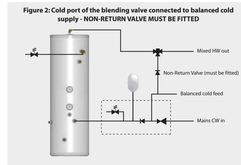
The diagrams opposite shows how the blending valve can be piped onsite.
