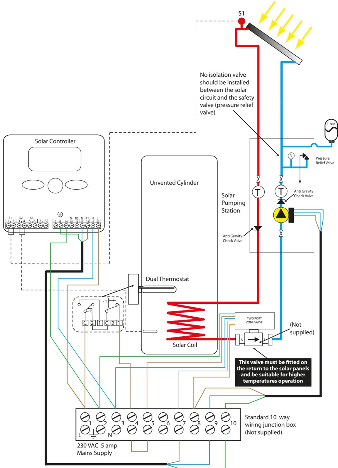
(S-PLAN) WIRING DIAGRAM WITH TWO 2 PORT VALVES
