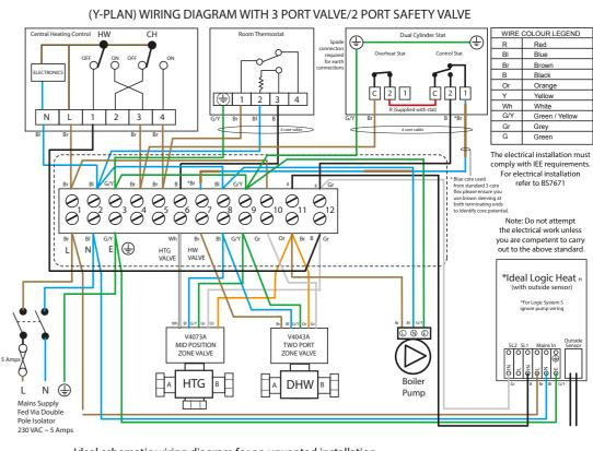
Ideal schematic wiring diagram for an unvented installation
