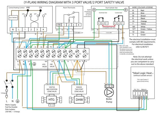
Ideal schematic wiring diagram for an unvented installation
