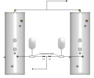
If two Thermstore cylinders are coupled together the secondary inlet and outlet pipes must be balanced. The units must be fitted on the same level.
