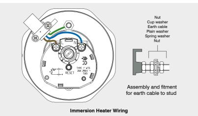
Thermostat Type WTS fitted in the immersions, and are supplied set in position 4.5 at  $61^{\circ}C \pm 3^{\circ}C$ .
