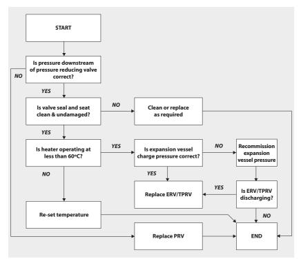
FAULT - Water Discharge Into Tundish
