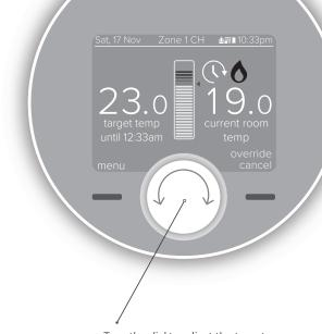
Turn the dial to adjust the target temperature temporarily (this could be up or down)
